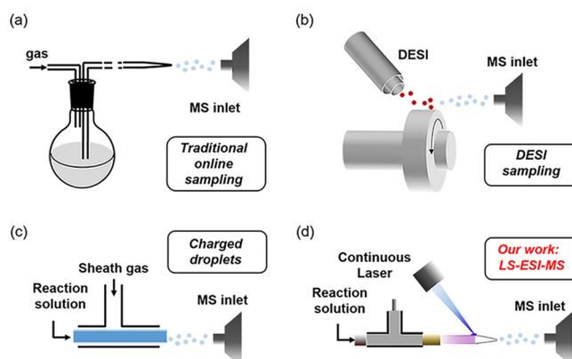
**Figure 1.** Comparison of (a) traditional online PSI MS; (b) direct detection of short-time reaction using in situ DESI MS; (c) microdroplets' acceleration; (d) our work: LS-ESI-MS.
